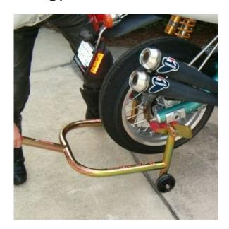
The swivels should be placed as shown below, with the rearmost peg <u>behind</u> the swingarm, not underneath it. The counterweight will ensure that the swivels are in the proper position to lift your motorcycle.
