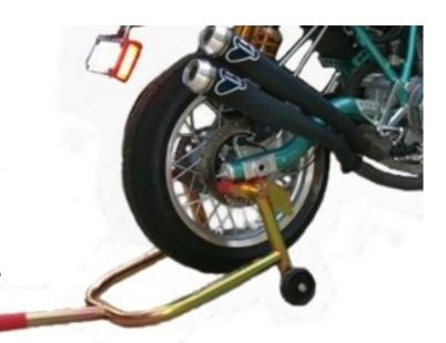
When lifting the motorcycle, place one hand on the stand and with the other hand hold your motorcycle upright while you line the stand up and complete the lifting process.
