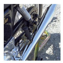
Use the 3/8 - 24 x 2-3/4" bolt and the thin hex nut on the left side.
