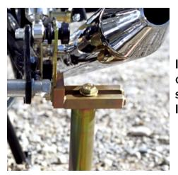
Use the 3/8 - 24 x 2-3/4 bolt and the Nylock nut on the right side.
